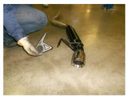
2) Place a provided 3" clamp onto the expanded end of left mid pipe **#26514S**, then slide completely onto the left side of the Scavenger assembly and tighten the clamp enough to hold, but still allow for adjustment. Repeat this step on the right side of the vehicle with mid pipe **#26515S**.
